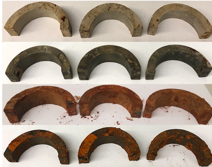
Fig. 2. Coupons after 400 hr of exposure prior to cleaning. Black, brown and grey types, left to right. Dissolved oxygen (top row). Peracetate-singlet oxygen (second row), chlorine dioxide (third row), peracetic acid (bottom row).
